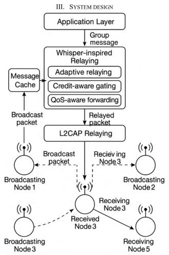
This section presents the design of a peer-assisted broadcast framework that adapts the Whisper Protocol's low-redundancy flooding principles to the Bluetooth Low Energy (BLE) stack. The system uses L2CAP Connection-Oriented Channels (CoC) for structured, flow-controlled communication and enables scalable, low-latency group broadcasting through partial mesh topologies and probabilistic peer relaying.
